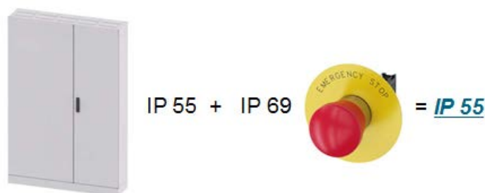
Figure 6-75 Example: Alteration of the degree of protection by installation of a component
